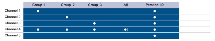
The table shows an example of how **NIROS RX8008 PLUS** on one or several channels is adjustable between different types of calls or combinations of calls. This eliminates the risk of an incorrect set-up of the alarm receiver.
