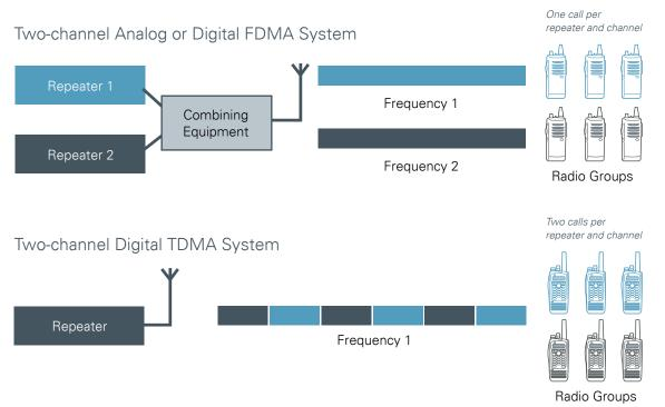
TDMA-based systems also offer the flexibility to adapt as new applications emerge to make additional use of the two time slots — preserving initial investments while providing an open path to future usage models for digital two-way radio. For example, the future roadmap for two-slot TDMA applications includes the ability to temporarily combine slots for increased data rates, or to use both slots together to enable full-duplex private calls.
